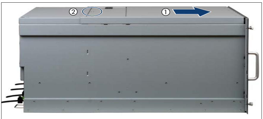
Figure 8: Installing the front cover
